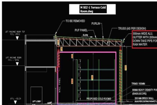
Rainwater Collection Piping/Gutter System for M SEZ-1 terrace
