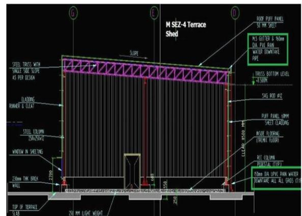
Rainwater Collection Piping/Gutter System for M SEZ-4 terrace
