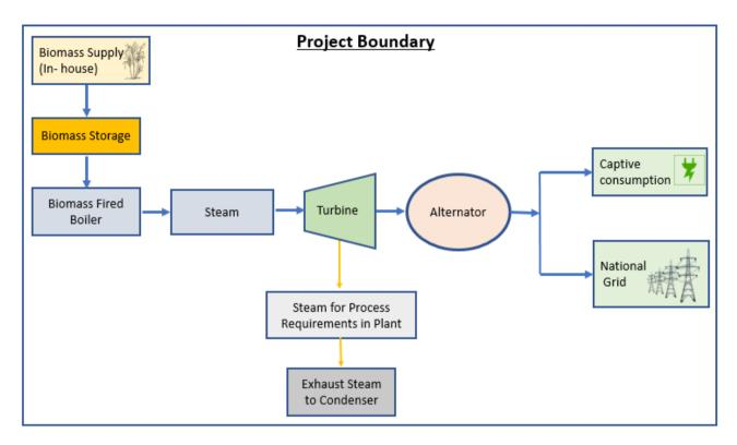
The project activity involves generation of renewable electrical energy from the combustion of renewable biomass, to generate process steam and electricity for captive consumption and grid supply. The technology employed is a biomass-based cogeneration system, generating steam and electricity. Thus, the technology to be used in this project is indigenous and is environmentally safe & sound. Emission reductions will be claimed from electricity exported to grid only.
