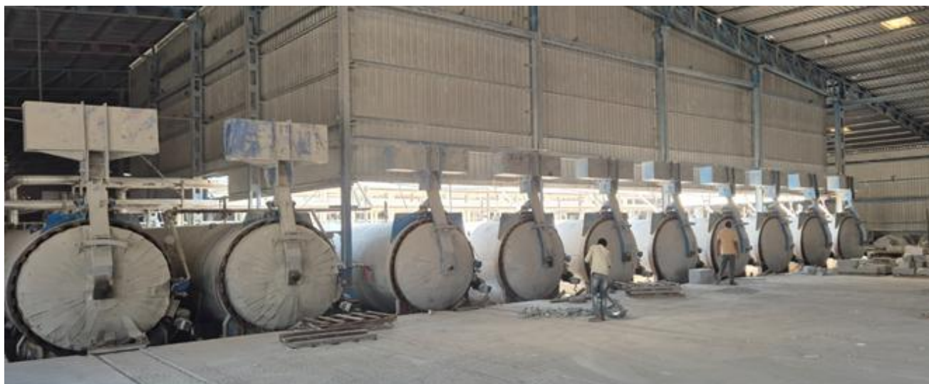
Figure 6 Steam Curing Process (Autoclave Reactor)
